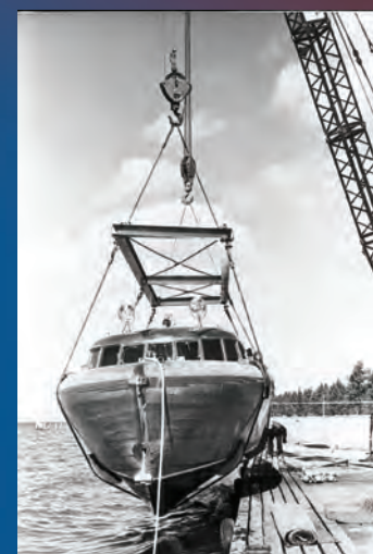
Harrah replaced the Kermath engines with Allison's, changed the configuration, and added the deck house flybridge superstructure.
